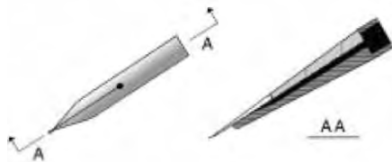
fig. 2.5. Essential construction of a pen
