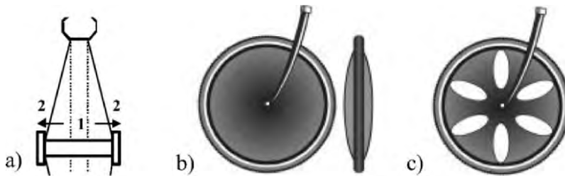
fig. 15.18. Disc-diaphragm-wheel: construction (a), normal (b) and light-weight (c)
