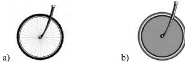
fig. 15.17. Alternative systems: spoke (a) and disc wheel (b)
