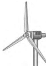
fig. 11.9. Wind power plant with horizontal rotation axle
