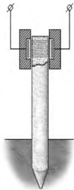
fig. 9.17. Piling with electrodynamic movement
