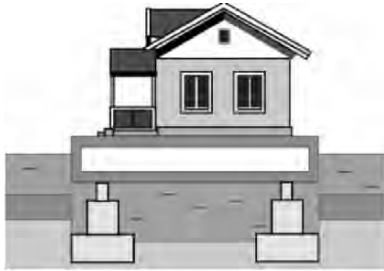
fig. 6.6. House on pontoons and on moveable pillars
