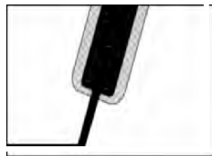
fig. 2.7. Basic construction of a felt-tip pen
