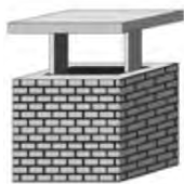
fig. 11.14. Cover of a chimney
