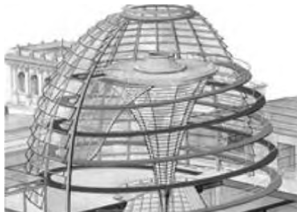
fig. 9.20. Ramps to the visitor's platform in the dome of Reichstag (Germany's Parliament building) in Berlin
