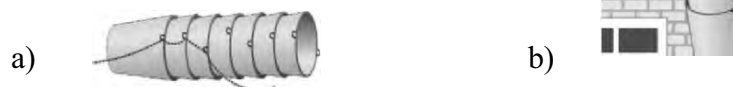
fig. 6.9. Tube for construction waste removing during transport (a) and during work (b)
