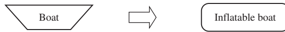
Figure 11.30 Principle 29—Pneumatics and hydraulics. Use gas and liquid instead of solid parts.
