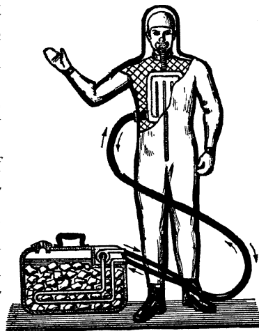
Figure 9. Extraction Principle: Rescue workers carried backpacks containing cooling devices; now these devices are placed in a separate container.
