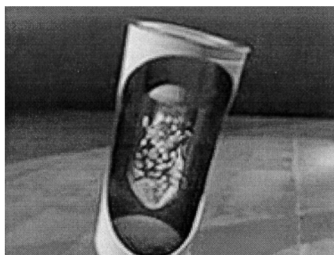
Draining of the water onto the CaO
