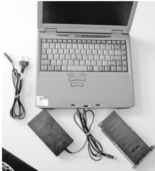
Figure 2. Notebook computer with two systems of power supply
