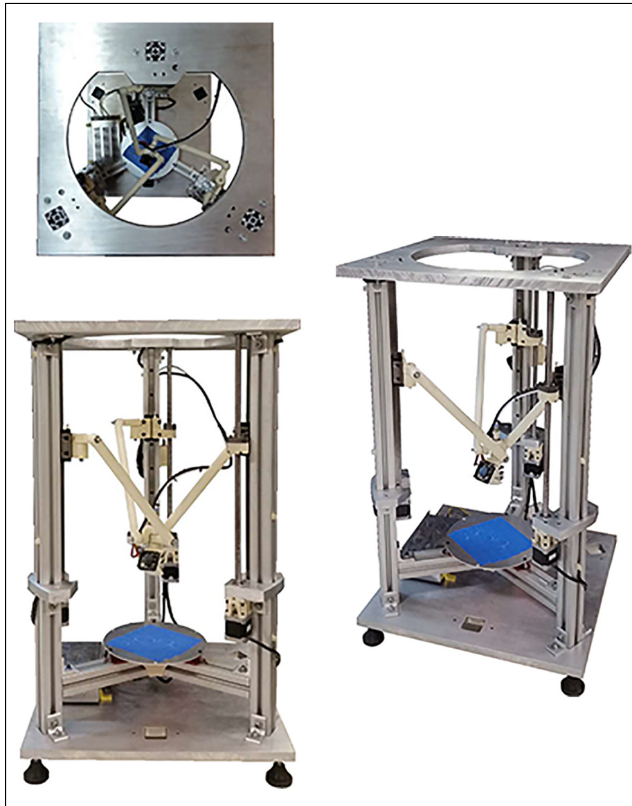
Figure 11. The fabricated aluminum prototype of the LDr-AM.
