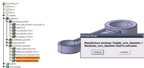
Figure 8 Manufacture problem in forge
