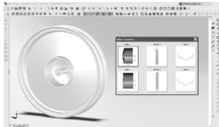
Figure 4 Customization of a moped wheel by using geometrical models DB.
