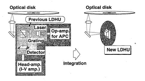
Fig.1. Previous and New Optical Pick-up by Matsushita Electronics Corporation (Proceeding from an oral presentation on IEEE ISSCC '96 in San Francisco )
