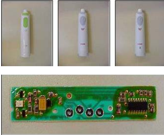
Figure 5. Housing unit and printed circuit board
