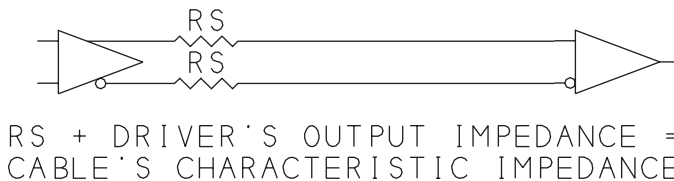
Figure 7-7: A series termination can absorb reflections.
