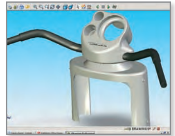
Image 4: CAD illustration of gauge pod.
