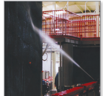
Image 2: Pressure-testing a working prototype at 100 psi
