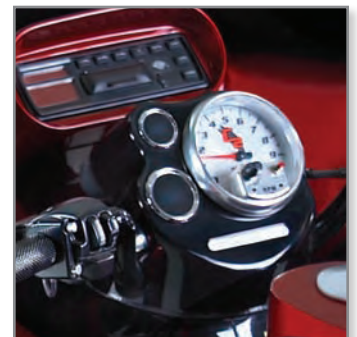
Image 3: Painted polycarbonate gauge pod installed directly on the bike.
