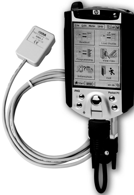
Fig. 1–33. Example of a data collection and analysis device for metering purposes. (Photo courtesy of Iskraemeco.)
