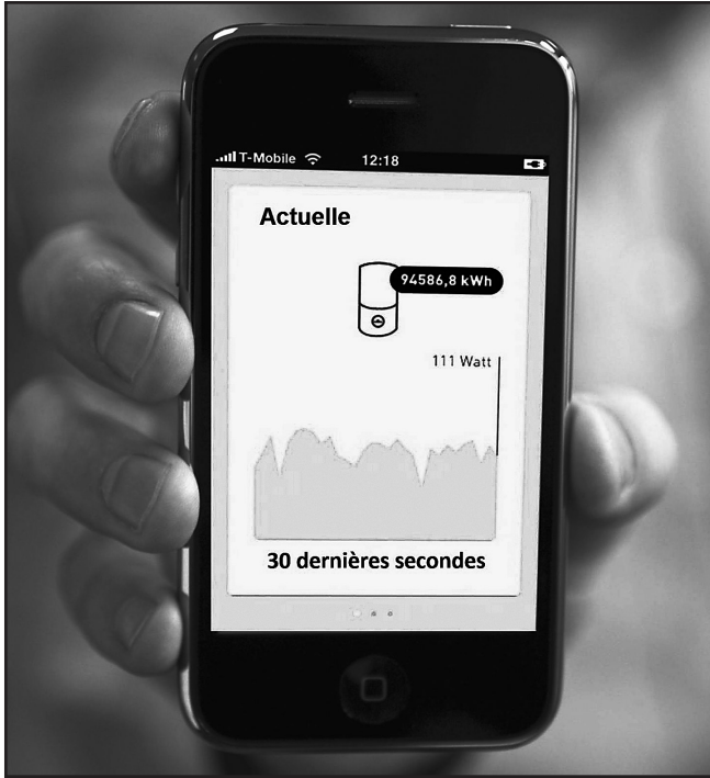
Fig. 3-5. A smart metering system integrated with a modern customer displays on a mobile smart phone. (Photo courtesy of Yello Strom.)
