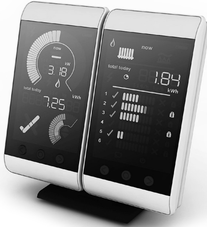
Fig. 2–34. Example of a customized display device. (Photo courtesy by Green Energy Options.)
