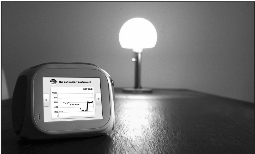
Fig. 3-6. An example of a smart metering system integrated with modern customer displays on a Chumby device. (Photo courtesy of Yello Strom.)
