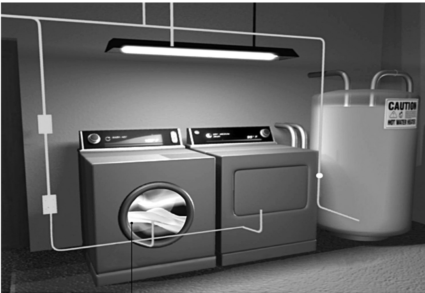
Washer signals requirements directly to water heater.
