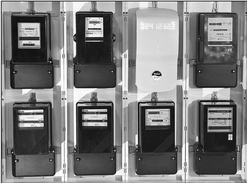
Fig. 2-1. Example of electromechanical meter registers versus a modern customer display unit. (Photo courtesy of Yello Strom.)
