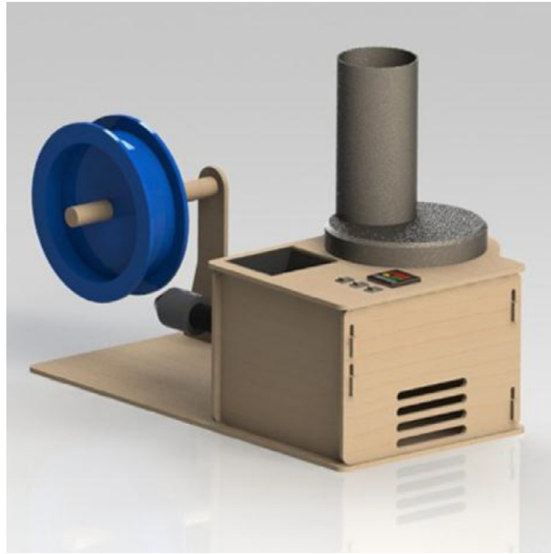
Figure 10.17 The Filabot recycling machine.
