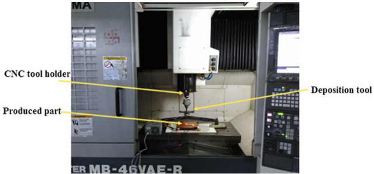
Fig. 9 Material deposition tool mounted on CNC milling machine
