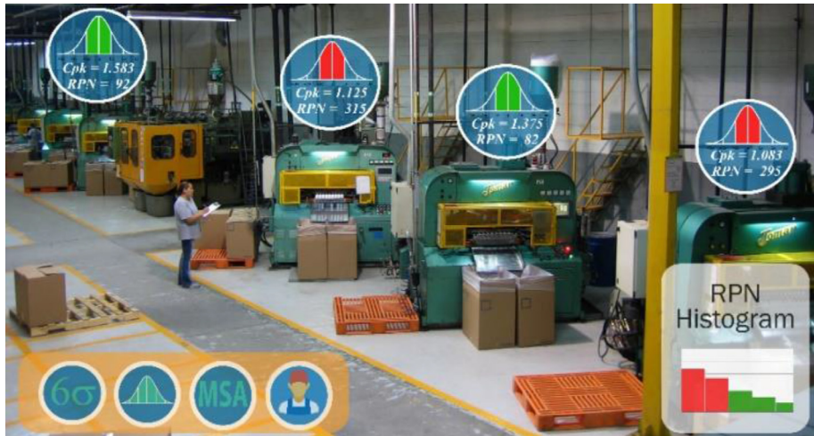
Fig. 13. Conceptualization of using the AR-QDA application on a full productive line [83].
