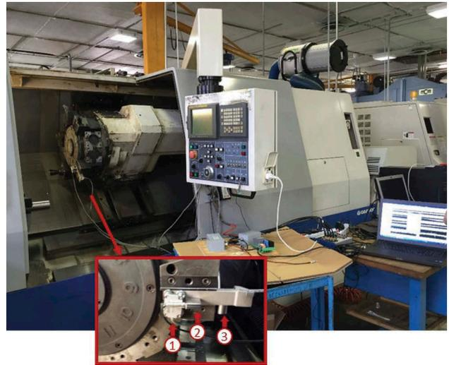
Figure 2. Multiple sensor monitoring system for smart monitoring of turning processes.
