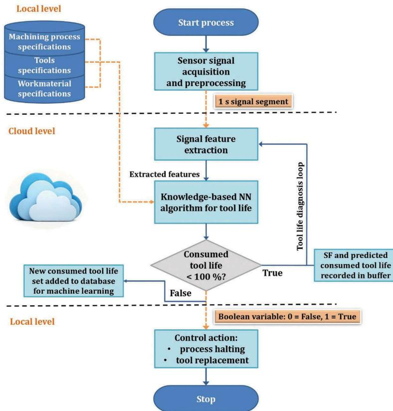
Figure 4. Workflow of the NN-based consumed tool life diagnosis procedure.
