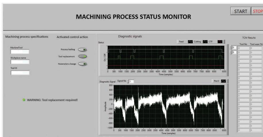
Figure 5. Machining process status monitor on the local terminal.
