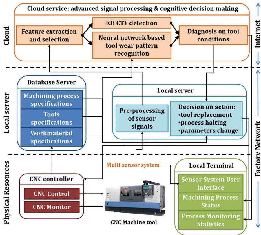
Figure 1. Architecture of the cloud-based cyber-physical system for smart monitoring of machining processes.
