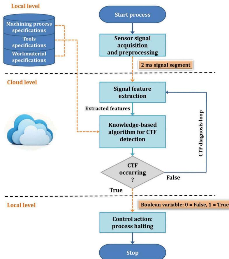
Figure 3. Workflow for online knowledge-based CTF detection procedure.
